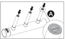
Keep Construction Caps in Risers (A) so Manifold remains clear of debris during construction
