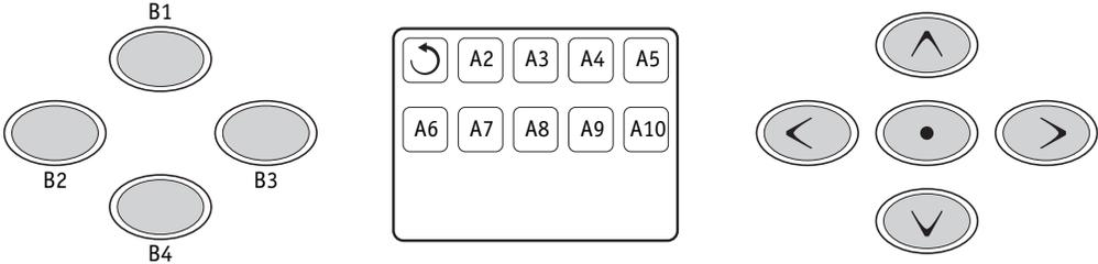
**Note:** Button B2 is ALWAYS unused on TP800 when used with this sytsem. A custom overlay will be required.
