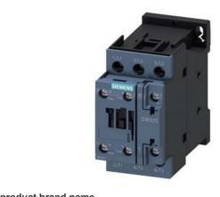
Power contactor, AC-3 32 A, 15 kW / 400 V 1 NO + 1 NC, 230 V AC, 50 Hz 3-pole, size S0 screw terminals Upright mounting position
