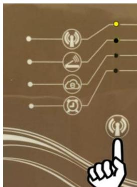
On the Wi-Fi module press the signal button, once the yellow light at the top is on you have successfully switched to AP mode.
