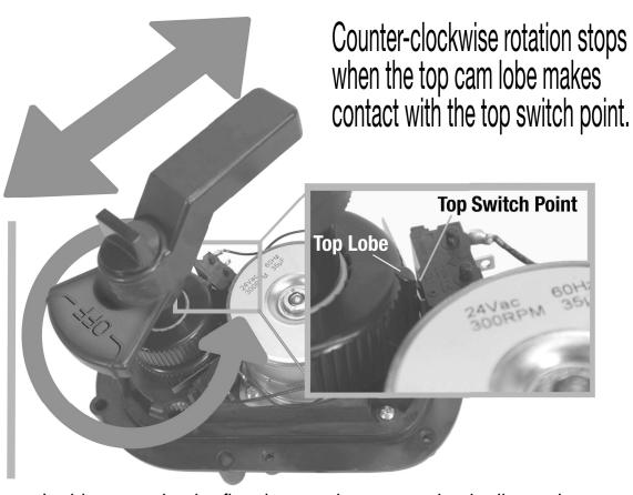
In this example, the flow has not been completely diverted at the stopping point.
