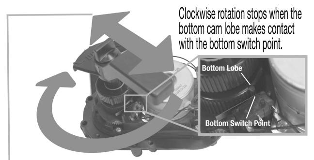
In this example, the flow has not been completely diverted at the stopping point.
