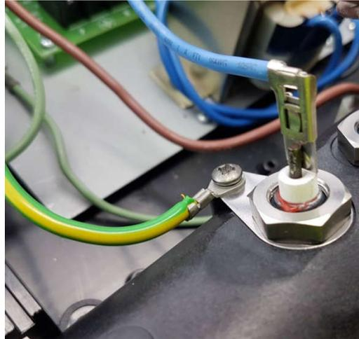
15. Connect the element brown active wire from the heater relay to the vacant connector on the thermal overload of the new element.
