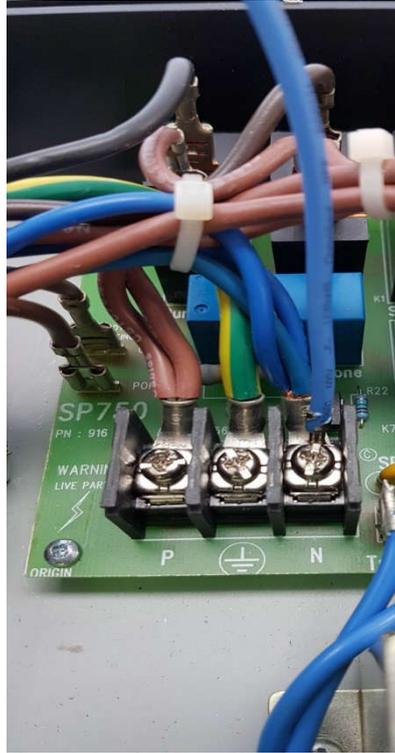
18. Position the black water sensor cable underneath the other wires so that it cannot be damaged when the element is laid flat. Plug in the new water sensor plug onto the circuit board.
