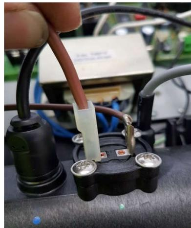
16. Connect the brown wire from the element wiring to the POH1 connector on the circuit board.
