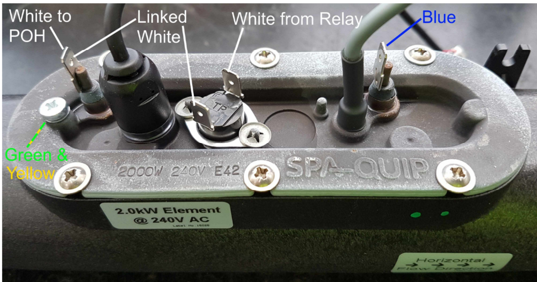
Incoloy Heater Element pre Nov 2015 wiring connections
