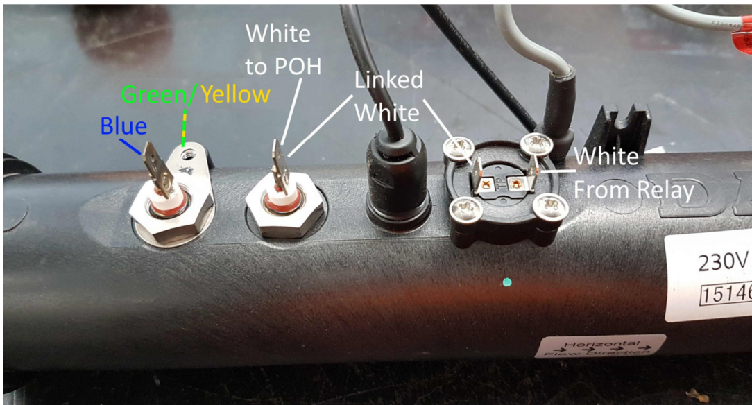
Titanium Heater Element pre Nov 2015 wiring connections
