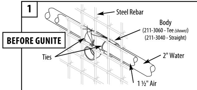
1. Hang Power Gunite Jet Body with ties through preset holes onto steel rebar.
