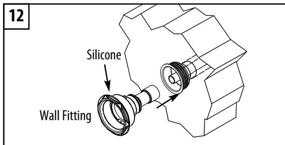
12. Put a bead of clear silicone sealant all around the back side of the wall fitting's flange. Prime and cement the end of the 1" pipe and fitting socket. Slide fitting onto end of 1" pipe until tight against the plaster niche.
