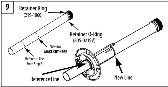
9. Remove the 1" pipe assembly from the jet body assembly and realign the measuring tool with the reference line. Make a new line at the Power Storm Gunite Jet setback on the measuring tool.
