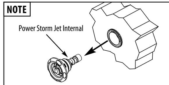
Note: To winterize the jet system, unthread the jet internal from the wall fitting ONLY. Install a #10 rubber expansion plug inside of the fitting opening.
