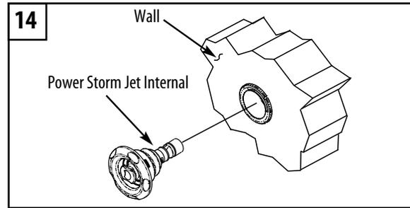
14. Insert Power Storm Internal into the wall fitting and thread in passed first stop. Do not force. To reduce water flow, turn clockwise. To increase water flow, turn counter-clockwise until it stops turning. To remove, continue turning counter-clockwise past the stopping point. You will hear a snap to confirm release of Power Storm internal.
