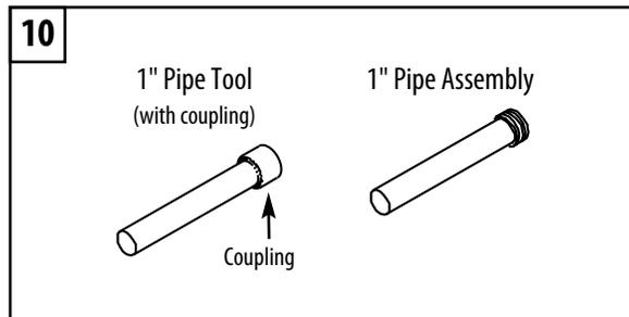
10. Create a 1" pipe tool with coupling attached to install the pipe assembly in the following steps.
