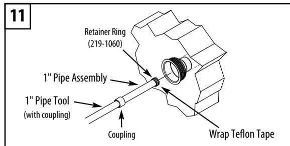
11. Install 4-6 wraps of Teflon tape around the threaded Retainer Ring, including 1 wrap over the o-ring. Dry fit the pipe tool with coupling on the end of the 1" pipe assembly. Thread the assembly into the body assembly until it is snug and the pipe tool with coupling spins freely. Remove the pipe tool from the end of the pipe assembly.
