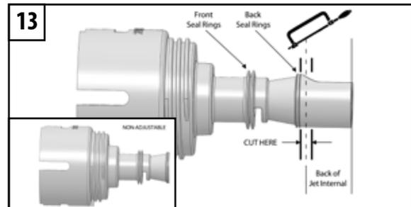
13. To make a non-adjustable jet internal, cut off the back of the jet internal after the back seal rings.
